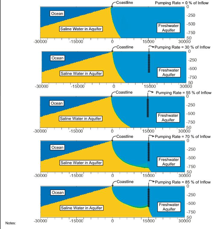
Series of images depict cross-section view of a coastal margin aquifer showing equilibrium salinity distribution for a range of pumping rates. Pumping is 15000 feet inland from the coastal margin.
